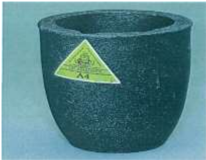
Figure 1. Crucible used in Melting of Aluminium.
