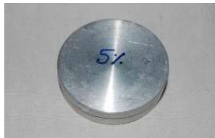
Figure 4. Specimen with 5% Quartz composition in Aluminium Quartz composite.
